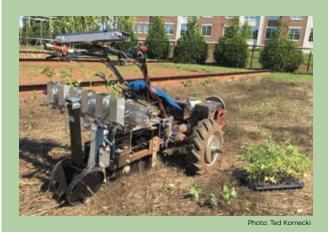
No-till transplanters such as this one designed for a walk-behind tractor can make reduced tillage vegetable systems more efficient.
