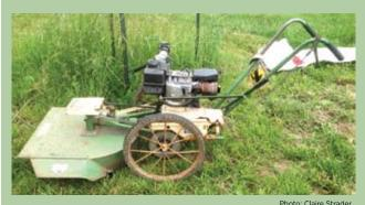
A walk-behind rotary mower is especially useful for managing living aisles.
