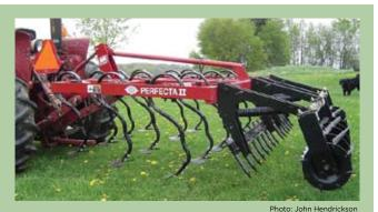
This Perfecta field cultivator can prepare ground for seeding cover crops and can be used to lightly incorporate broadcast seed.
